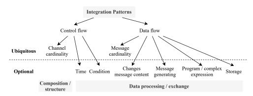
Figure 4: Categorizing integration pattern characteristics according to control and data flow
