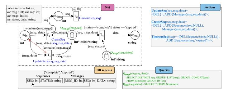
Figure 8: Timed db-net realization of an aggregator
