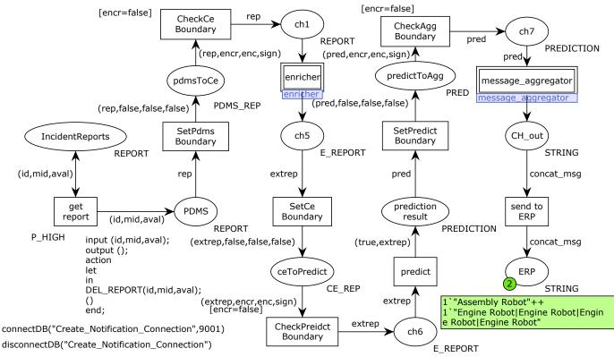
Figure 41: Predictive maintenance scenario simulation
