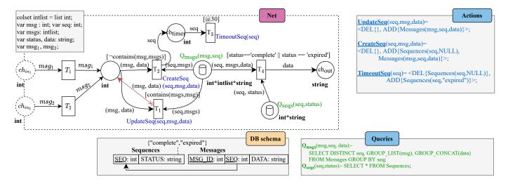
Figure 10: Sequential composition of timed db-net realizations of a join router and an aggregator
