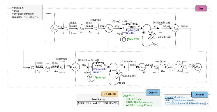
Figure 37: Material replicate scenario as a timed DB-nets with boundaries
