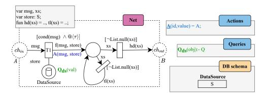
Figure 15: Interpretation of a message processor pattern.
