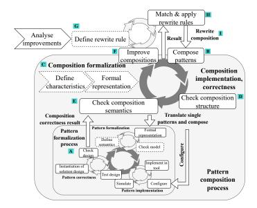
Figure 2: Responsible pattern composition and optimization process (white colored boxes denote the main steps, grey colored box shows the *pattern formalization process* from [6], to which we bridge through translation of single patterns and compositions)
