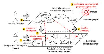
Figure 1: End-to-end perspective from integration process modeling to verifiable execution semantics and automatic, correctness-preserving improvements (current gaps or missing aspects in red color).
