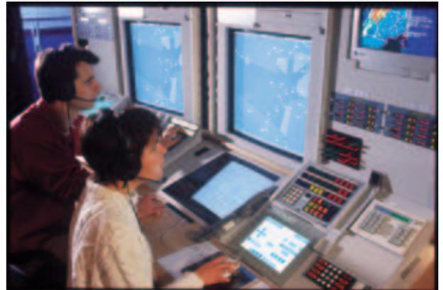
Figure 2: ODS control working position
