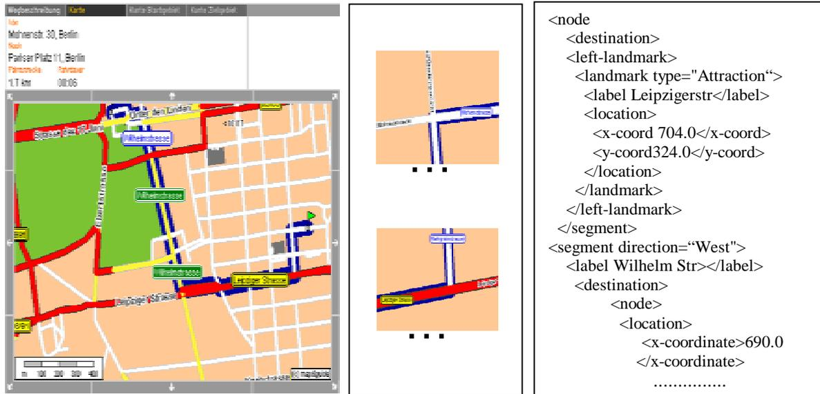
Figure 4. Analyzing a map in order to construct a symbolic description (here in XML format) of the core contents (here a route description).
