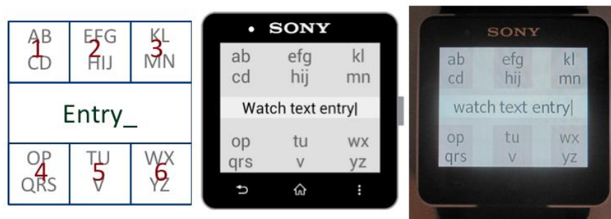
Figure 1. Our prototype implementation on a Sony SmartWatch 2: (a) concept, (b) design, and (c) implementation.
